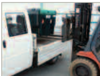
TRUCKMASTER BEING LIFTED USING SPECIFICALLY DESIGNED FORKLIFT SLOTS ON THE BASE
